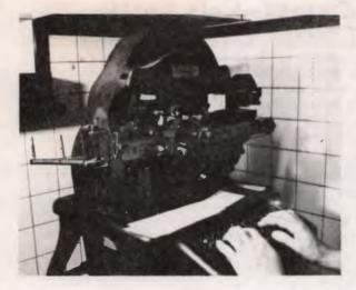
This is a Graphotype machine, a component of the Party's automated mailing system. The Graphotype makes an address plate which is used in another machine to instantly address a piece of mail. The plates made by this machine resemble minature license plates which contain your complete name and address. All of these plates are kept in a safe place under double lock.
